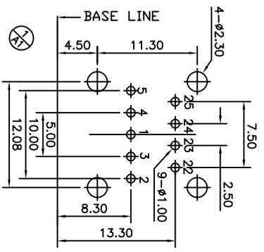
**RECOMMENDED PCB LAYOUT(PCB THICKNESS: 1.6mm)
